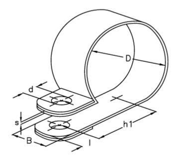
$\begin{array}{ll} d & = 10.5 \\ Diameter D = 16 \\ h1 & = 22.5 \\ I & = 10.0 \\ s & = 1.0 \\ Width B & = 25 \\ \end{array}$
